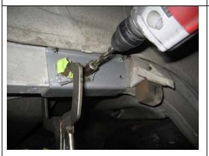
Drill the 3/8 inch holes through the frame using the channel bracket as a guide. Using the drill guide the front hole will be drilled from inside the frame rails (the snubber bracket is in the way on the outside) and the rear hole is drilled from outside the frame rail because the floor interferes with the drill motor on the inside.
