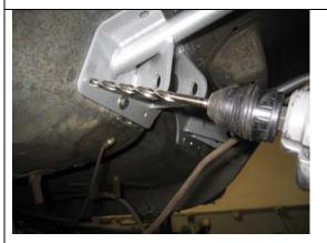
Finish drilling the remaining 10 holes with the two alignment bolts holding the cradle secure.
