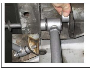
The rear axle assembly needs to be installed next to determine the correct location for the upper bar tabs to be welded on the housing.
