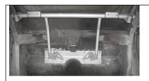
Swing the cradle up to the angled tunnel/floor pan area in front of the pinion snubber bracket. Remove any tabs or brackets (brake line tabs, etc.) that will interfere with the folded front plate of the cradle from setting flush with the tunnel/floor pan area
