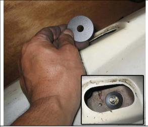
Install the large thick washer onto the bolt through the shock hole inside the trunk area. Install nut and tighten.
