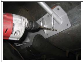
With the cradle seated securely up against the tunnel/floor pan area and centered between the frame rails use the center hole in the cradle as a guide and drill a 5/16 inch hole through the hole. Install a 5/16 inch button head bolt to maintain alignment while drilling remaining holes. Repeat on other side.
