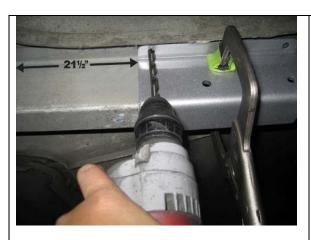
Install the cross-member frame saddle brackets onto the frame rails just behind the axle snubber brackets with the angled end forward and the square end towards the rear. Double check the location by measuring from the top folded edge of the bracket back to the front edge of the stock rear spring shackle tube that sticks through the frame rail. The reference measurement is:
