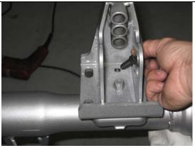
After both sides are drilled rotate both brackets 180 degrees and install the Allen bolts and tighten.
