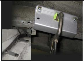
Install the button head Allen bolts with washers through the sandwich brackets, the floor and the frame channel brackets and secure with nuts.
