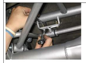
Install the sway bar brackets on the cross-member brackets that support the sway bar. Install the nuts onto the bracket bolts and tighten. Once the brackets are tightened, the sway bar has to be centered. Rotate the bar up where it is between the frame rails and measure from the end of the bar to the inside of the frame and slide the bar either way until that measurement is equal. Slide the lock rings tight against the flange on the urethane and tighten set screw.
