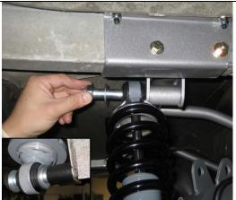
The coil-over shocks are installed next. The top bolt is 5 by 5/8 inch with a washer on the outside of the urethane bushing and the bottom bolt is 6 by 5/8 inch with washers on both sides of the urethane bushing with a 1 3/8 inch spacer between the washer and the bracket.
