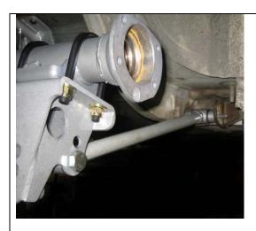
Next position the rear of the lower bar into the bottom hole on the axle bracket and install the 3 by 5/8 inch bolt.
