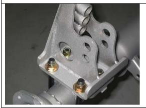
Rotate the brackets back to their correct location and install the Allen bolts and the u-bolts and finish tightening.
