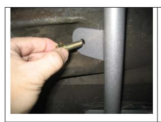
Install the 3/8 inch bolt through the tab on the cradle through the stock shock hole.
