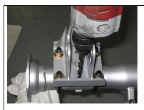
Drill a 3/8 inch hole through the spring pad using the hole in the axle bracket as a guide. Repeat the process for the other side.
