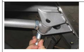
Adjust the top bars need to 13 7/16 inch centers and the adjustor end installed in the brackets on the cradle using the 3 by 5/8 inch bolt.
