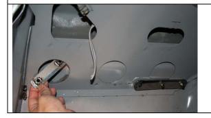
The lower sandwich plate is installed as pictured. The inside plate with the weld nuts will have to be slid through the side hole as pictured and aligned over the drilled holes above the lower sandwich plate and the bolts tightened from under the car. The button heads used on the weld nut plates are 5/16 coarse by one inch.
