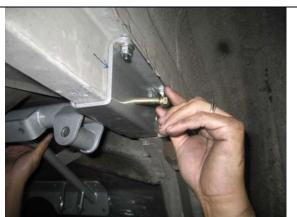
Lift the cross-member cradle between the channel brackets aligning the rear cross-member flange hole with the rear hole in the channel bracket and install the  $3/8 \times 3$  inch bolt from the outside. Lightly tighten.
