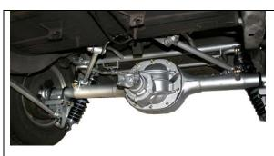
Finish tightening all the bolts including the jam nuts on all four adjustors. You are ready to install the drive shaft and set the car on the ground.
