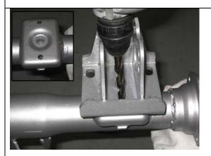
With the axle bracket bolted down and using the axle bracket as a guide drill the remaining hole in the spring pad.
