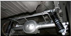
The rear height of the car can be adjusted by loosening the set screw in the lower shock ring and turning the ring with a spanner wrench. The car needs to be raised up in the rear to relieve the weight off the shocks to turn the lower ring.
