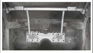
Cross-member cradle assembly completely installed.
