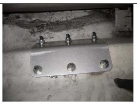
After all the holes are drilled remove the two alignment bolts and install the two folded sandwich plates over the drilled holes in the trunk area with the notch on the plate facing down. Install the twelve 5/16 fine thread button head bolts and washers through the cradle, the floor pan and through the sandwich plates. Install washers and nuts and tighten.
