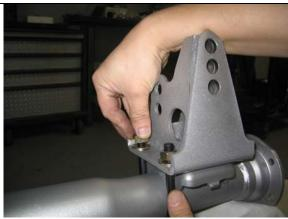
Bolt the coil-over axle bracket to the leaf spring pad checking that the center bolt on the bracket aligns with hole in the pad. If you have a different diameter center pin, use the old pin from your old leaf spring.
