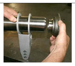
**Note:** If you are using a 9 inch Ford housing and welding on our coil-over axle brackets the bracket centers is 43 inches with the pinion down one degree from the back face of the axle brackets which are 90 degrees to horizontal.
