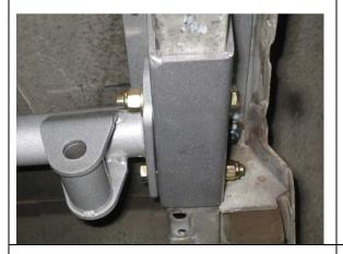
Install the two 3/8 x3 inch bolts in the front hole in the cross-member from the inside because of the snubber bracket issue. Tighten all four bolts.
